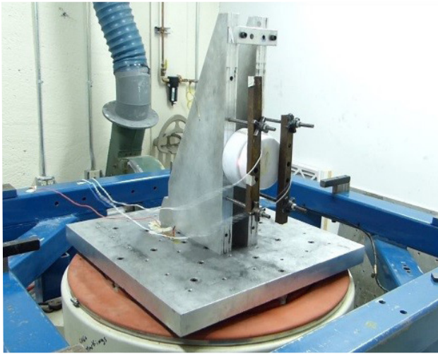
Figure 3: An AI product being tested to make sure it can withstand conditions like a rough ride in a pickup truck
